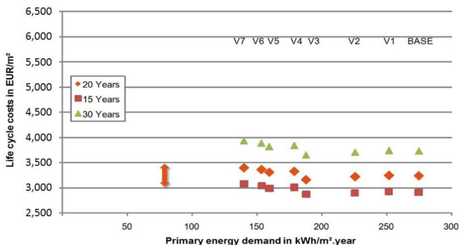
Figure 1. Results from the calculation of the life-cycle cost for different combinations of energy-saving measures using 3 different life times for the measures on a new office building. The cost-optimal level is not one point, but can be identified as a collection of equally good results, ranging from 225 to 180 kWh/m².year, depending on the energy-saving package variation.
