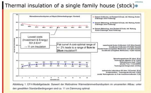
Figure 5. Calculated cost-optimal curve for a German single-family house.
