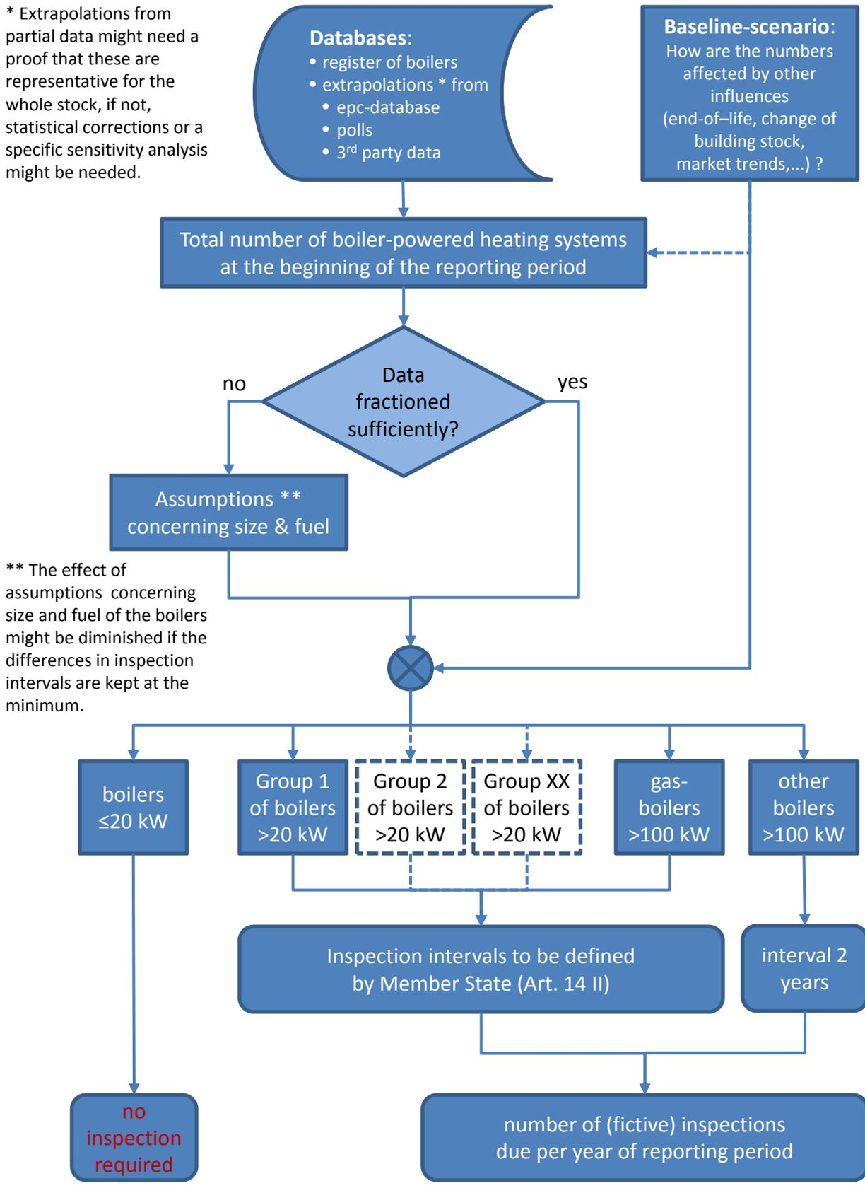
\*\* The effect of assumptions concerning size and fuel of the boilers might be diminished if the differences in inspection intervals are kept at the minimum.
